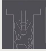
After understanding the condition of the plumbing, your technician may recommend hydrojetting, often referred to as jetting or hydroflushing. Hydrojetting is a quick, affordable method of removing waste, debris and blockages from your building's plumbing using a pressurized, continuous stream of water.
